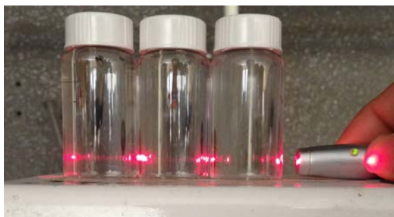
Fig 11. The Tyndall effect is shown above as light passes through (from left to right) solutions of butyric acid/water, butyric acid/ \text{MnSO}_4 /water, and butyric acid/ butanol/water.
