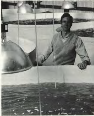
Jack Batchelder with 5,000-gallon tanks containing microscopic algae grown under powerful lamps. The algae is raised as food for each stage of the developing oysters and clams.
