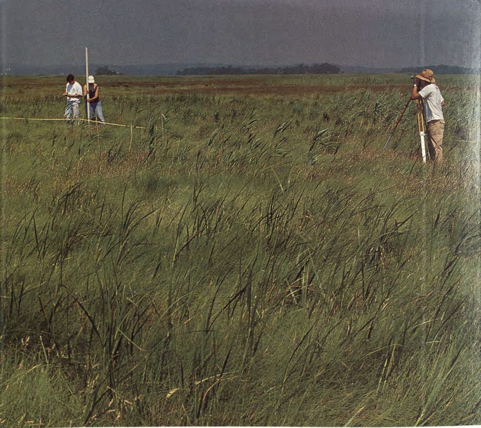
Above: Warren, at right, is assisted by Linda Reddington, RTC '95 and Ed Faison '95 to measure the elevation of a salt marsh. Note the band of phragmites in the background. Left inset: setting up a theodolite. Left below: Linda Reddington uses a cork dust gauge to measure the height of the last high tide. Undergraduate research assistants on The Phragmites Project: Mark Fallon '94; Ed Faison, Rachel Fertik, Stephen Fisk, Patrick Lee, Kristen Lennon, all the class of '95; Linda Reddington and Julie Zeppieri, both RTC students; Kate Newberry, Seth Weinstein and Sonja Weissbach, all class of '96.
