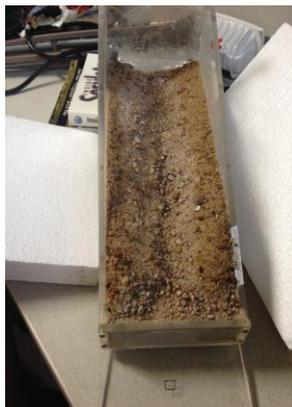
Figure 4.5b: Darkening of surface along the central channel, bottom of slope, and sides of box after 20 minutes of second thawing cycle.
