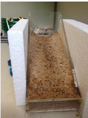
Figure 4.5a: Darkening of surface regolith after 45 minutes occurring down the length of the central linear depression and across the width at the bottom of the box.
