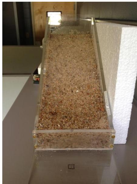
Figure 4.2a (left): Darkening of regolith beginning at the bottom of the slope after 60 minutes of thawing.
