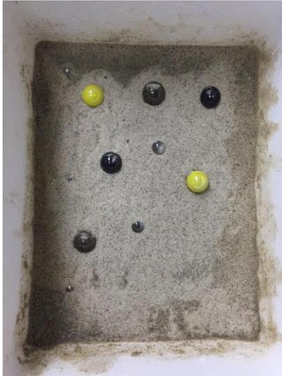
Figure 4.16c: Wetting of the regolith extending from the sides of the box after 90 minutes of thawing
