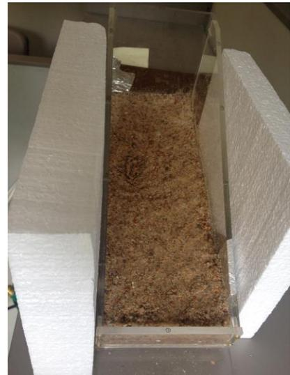
Figure 4.1c: Following three total hours of thawing, a small depression remains in place of the ice patch and additional darkening at bottom of the box.
