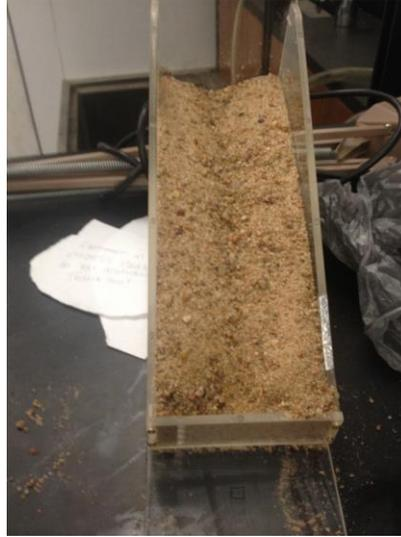
Figure 4.6a (left): Appearance of overburden and central valley in 4° C cold room at start of thawing.
