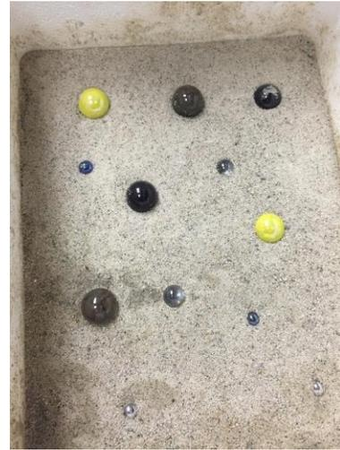
Figure 4.15c: After 24 hours of thawing, most significant association between wetting of surface regolith and marble placement is in the same location as in 4.15a and 4.15b.
