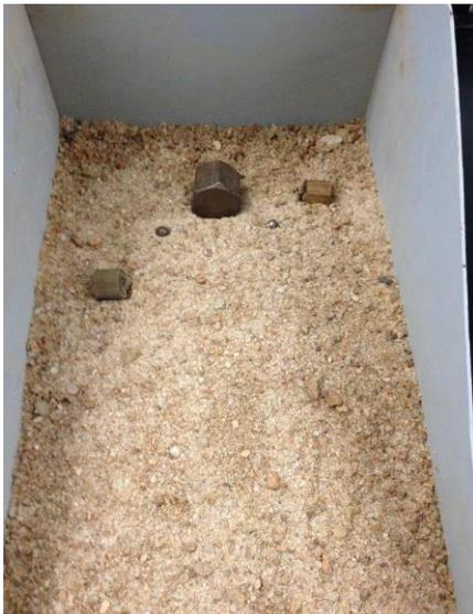
Figure 3.4: Metal hardware partially embedded in regolith to simulate boulder effects. Left to right: 1.5-cm light gold nut, rusted metal sphere (<1 cm), 2.5-cm dark metal cap, silver metal sphere, and 1.5 cm rusted metal nut.
