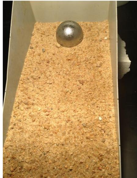
Figure 4.9: Thawing with the heat lamp in Experiment 2.5. Darkening can be seen in image at bottom of slope, and also was observed after 15 minutes of thawing in immediate contact with steel sphere at top of slope
