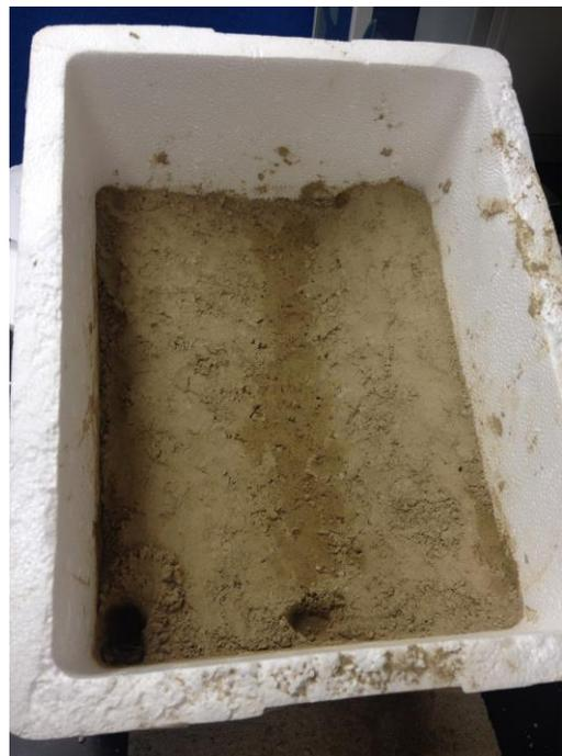
Figure 4.10: Dark linear feature extending down the central depression after nine hours of thawing on the 30° slope in the lab.
