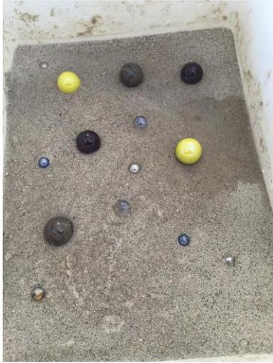
Figure 4.16a: Frozen, over-saturated regolith before addition of dry overburden layer.
