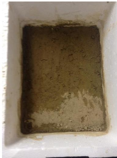
Figure 4.11a (left): Initial thawing began along the top of the slope and extended down both the sides and central swale.
