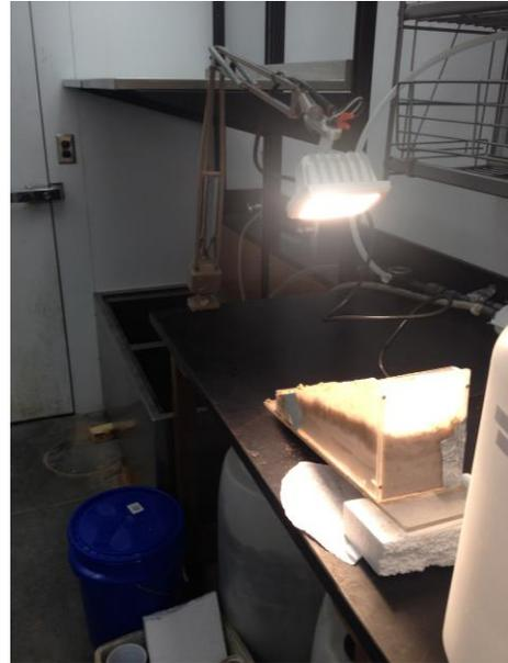
Figure 3.3: Thawing setup in the 4° C cold room with heat lamp applied approximately 30 cm from the surface.
