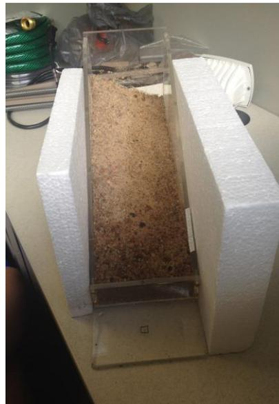
Figure 4.3b: Darkening of regolith observed in bottom right corner of box and slightly across width after 20 minutes of thawing
