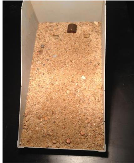
Figure 4.7: Patchy wetness throughout the surface regolith observed as darker areas after 30 minutes of thawing in experiment 2.2.
