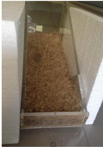
Figure 4.1b: Appearance after two hours of thawing with melting ice patch and darkening at bottom of slope.
