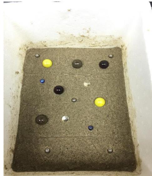
Figure 3.6: Marbles with 1.0-cm, 1.5-cm, and 2.5-cm diameters embedded in saturated regolith before freezing.
