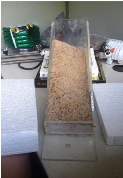
Figure 4.3a: Overburden regolith distributed in slope with deepest region on left side of box and low-lying region along right side
