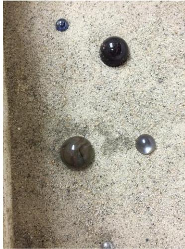
Figure 4.15b: Closer image of 2.5-cm marble after additional thawing in which dark regolith was both in contact with marble (bottom left side) and in surrounding area.
