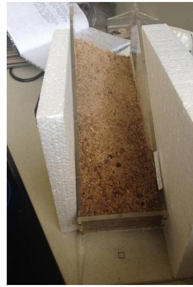
Figure 4.3c: After three hours of thawing, darkening of surface both across the width of the bottom of the box and extending in a linear trend along the right side of the box
