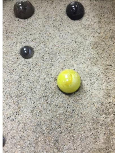
Figure 4.16d: Additional wetting after 90 minutes of thawing in direct contact with downslope side of 2.5-cm diameter marble
