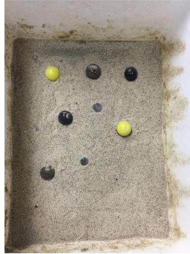
Figure 4.16b: System after addition of dry overburden layer at the start of the thawing cycle
