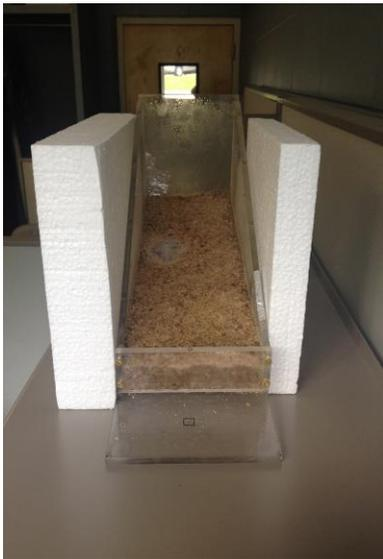
Figure 4.1a: Appearance of system at the beginning of the first thaw. Ice patch appears in top left of box.
