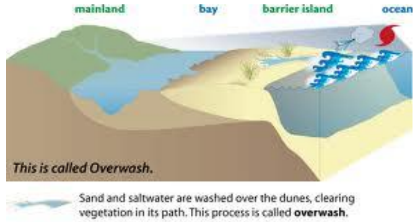
Figure 2.5: A diagram of a process called overwash, which occurs when a storm surge is high enough to overtop a barrier system (University of Maryland Center for Environmental Sciences).
