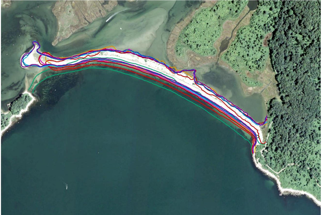
Figure 5.10: An image of digitized beach outlines representing locations from 1934 to 2014. The beach outline from 1934 is pictured in green , 1951 in red , 1968 in yellow , 1986 in pink , 1991 in maroon , 2010 in light blue , 2012 in dark blue and 2014 in purple .
