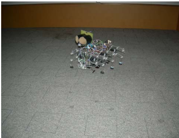
Figure 3. The photo of the predator with 2 light sensors, 3 SONAR sensors, and 2 antennas.
