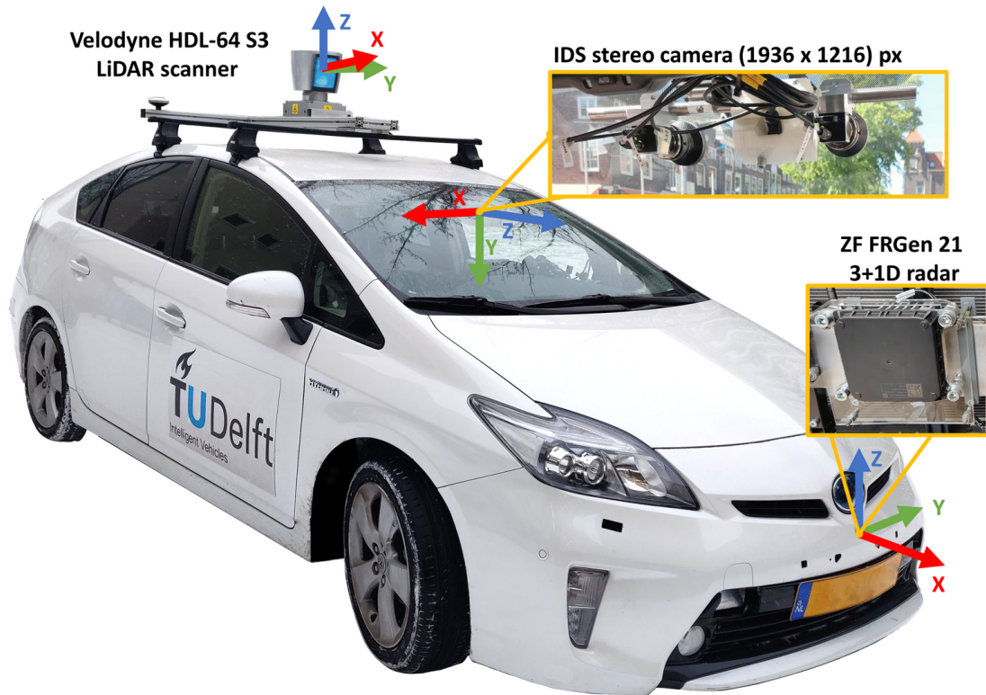
Figure 3.1: Vehicle and sensors used for the View of Delft dataset
