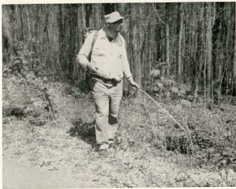
Fig. 3. Above: Back-pack sprayer of the type used in Region 7. Manufacturer's hose, wand, and valve assembly have been replaced by higher quality, better designed equipment. Side lever is on opposite side of tank in this view. Below: Back-pack sprayer in position for use. Lever is grasped by man's right hand.
