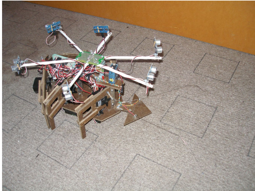
Figure 2. Photo of the prey with 6 range finding SONAR sensors and two antennas (wire touch sensors)
