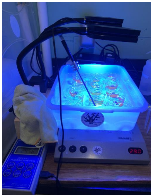
Figure 2. Stir bar exposure set up used for PE sphere and Brine Shrimp egg trials
