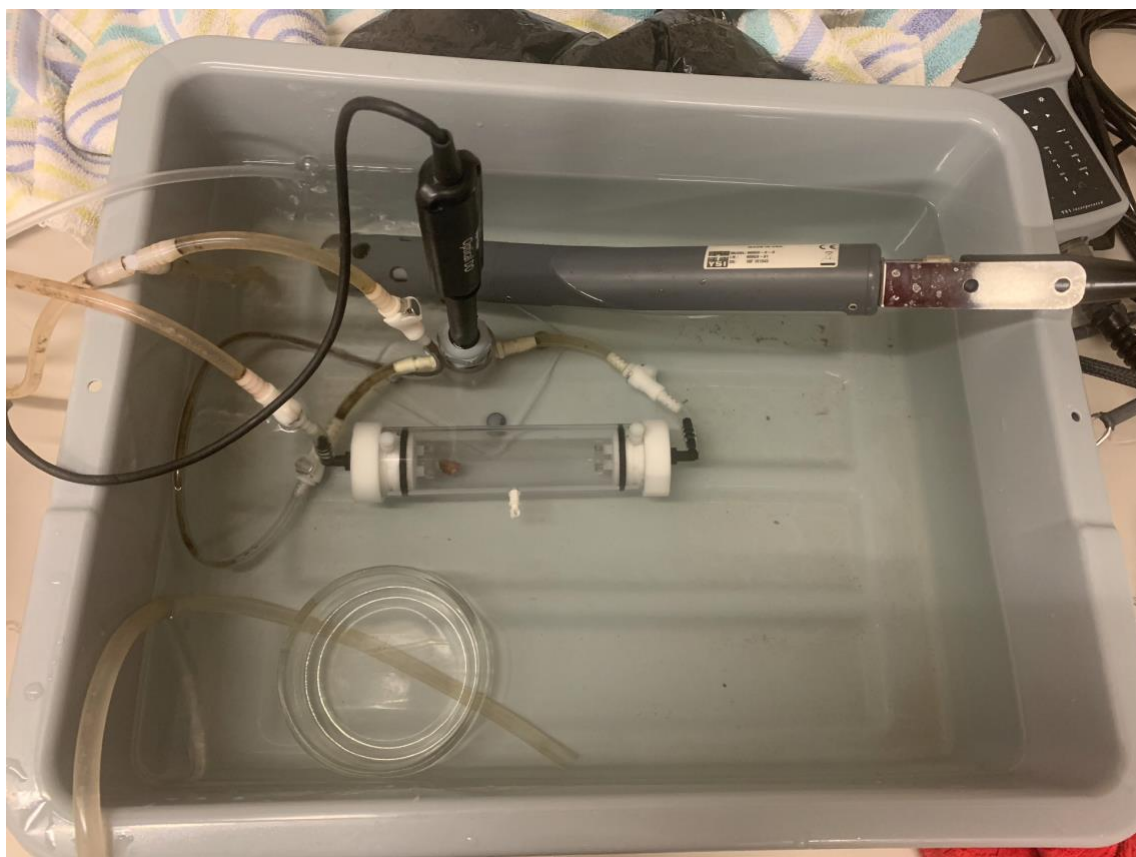
Figure 12. Respirometry set up with a colony in a chamber and water bath. YSI system is also pictured in the water bath, used for monitoring salinity and temperature.
