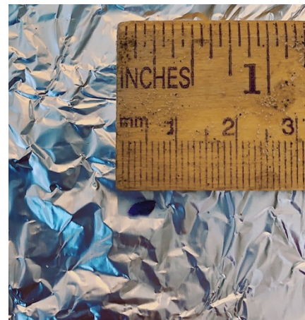
Figure 25: An image of sample BR1, which was a tiny purple rubbery pellet at the time of collection.
