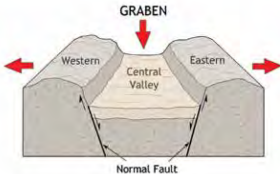
Fig. 6 Connecticut's Central Valley may have started to form as a graben but more rapid downward motion along eastern faults soon initiated eastward tilting of the valley's down-dropping metamorphic blocks.
