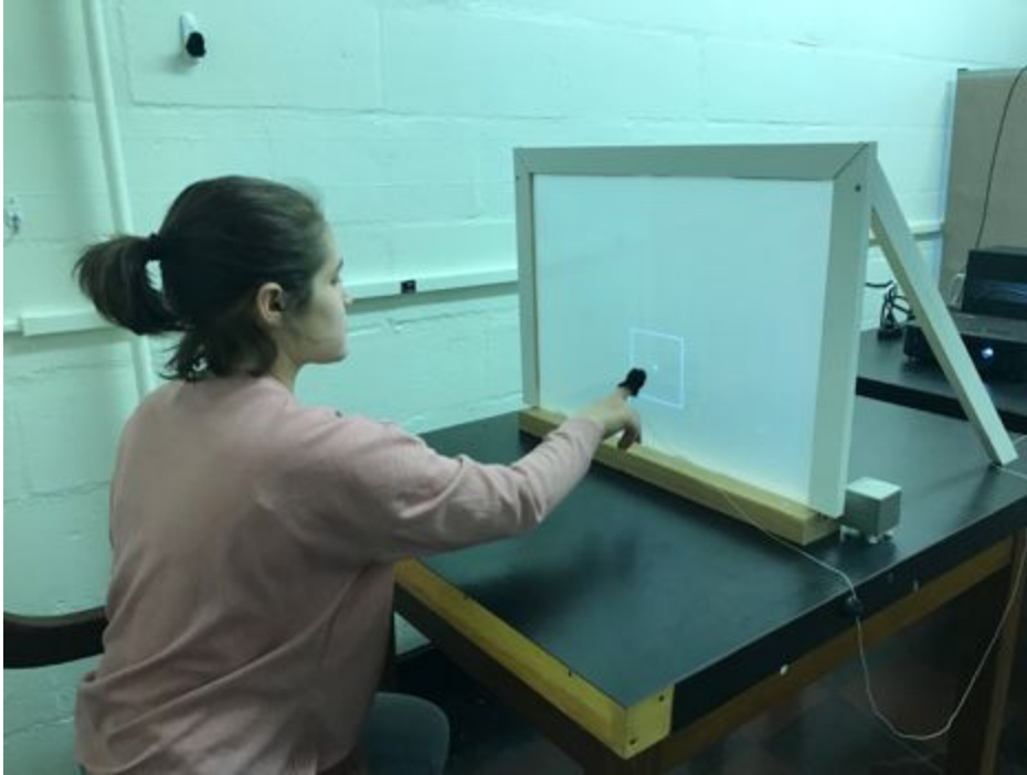
Figure 1. Lab setup of Experiment 1 and 2. The participant is wearing the sensor that helps to track the hand movements, and also was what allowed the images to advance when the participant swiped or tapped, similar to a touchscreen.
